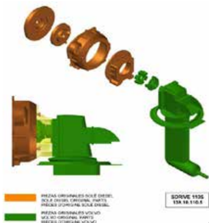
Solé Mini-17 + Volvo-Penta 120S sovite/adapter
